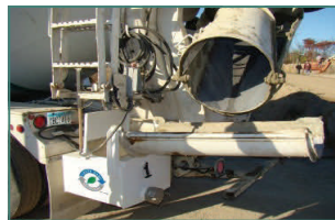
Chute washout box
